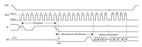
Figure 9.3 Read Identification (RDID) Command Sequence and Data-Out Sequence
