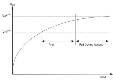
Figure 10.1 Power-Up Timing Diagram
